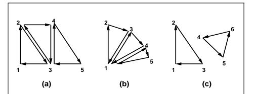
Figure 2.4. (a) A triangle strip. (b) A triangle fan. (c) Independent triangles. The numbers give the sequencing of the vertices between **Begin** and **End**. Note that the in (a) and (b) triangle edge ordering is determined by the first triangle, while in (c) the order of each triangle's edges is independent of the other triangles.
