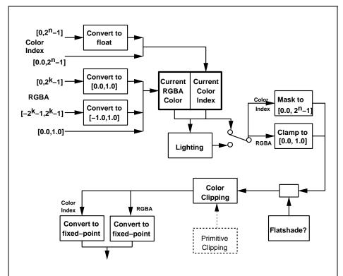
Figure 2.8. Processing of colors. n is the number of bits in a color index; m is the number of bits an R, G, B, or A component. See Table 2.4 for the interpretation of k.
