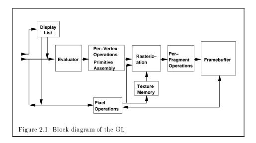
Finally, there is a way to bypass the vertex processing portion of the pipeline to send a block of fragments directly to the individual fragment operations, eventually causing a block of pixels to be written to the framebuffer; values may also be read back from the framebuffer or copied from one portion of the framebuffer to another. These transfers may include some type of decoding or encoding.
