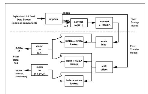
Figure 3.7. Operation of **DrawPixels**. The parameters controlling the stages above the dotted line are set with **PixelStore** while those controlling the stages below the line are set with **PixelTransfer** or **PixelMap**.
