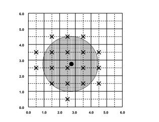
Figure 3.3. Rasterization of antialiased wide points. The black dot indicates the point to be rasterized. The shaded region has the specified width. The X marks indicate those fragment centers produced by rasterization. A fragment's computed coverage value is based on the portion of the shaded region that covers the corresponding fragment square. Solid lines lie on integer coordinates.
