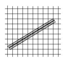
Figure 3.6. The region used in rasterizing and finding corresponding coverage values for an antialiased line segment (an x-major line segment is shown).
