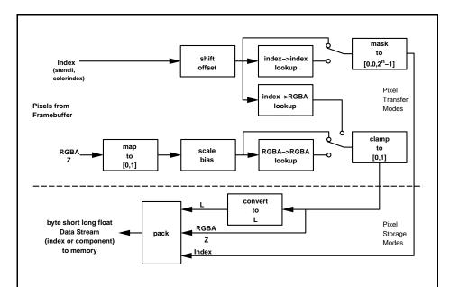
Figure 4.2. Operation of **ReadPixels**. The parameters controlling the stages above the dotted line are set with **PixelTransfer** or **PixelMap** while those controlling the stages below the line are set with **PixelStore**.
