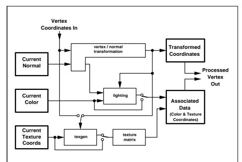
Figure 2.2. Association of current values with a vertex. The heavy lined boxes represent GL state.
